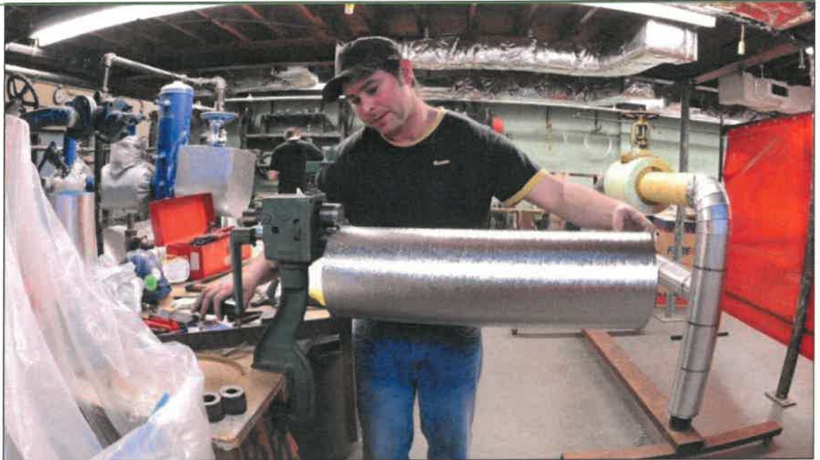
Apprentice Trevor Williams applying bead to aluminum jacket.
